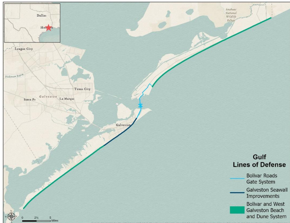
Figure 2-24. Gulf Lines of Defense of the Galveston Bay Storm Surge System
